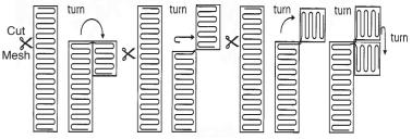
50mm minimal cable spacing
